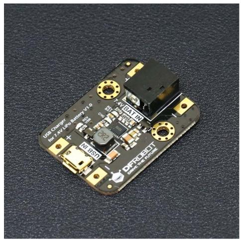
power bank) and an Android data cable, you can safely and efficiently charge the 7.4V lithium battery up to 1A, which commonly used in various robots and motor drivers. The light-weight and micro USB interface features make it ideal for outdoor applications. In addition to being a charger, it can also be embedded in a variety of 7.4V lithium battery-powered projects, adding a USB charging function to it, eliminating the need for battery swapping and the use of traditional bulky power adapters.
