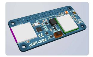
pHAT-GSM is a quad-band GSM/GPRS module that works on frequencies GSM850MHz, EGSM900MHz, DCS1800MHz and PCS1900MHz supporting GPRS class 12 data and Small-Message-System (SMS) functionality. Specifically designed for the Raspberry-Pi Zero user (can also be used on all the other Raspberry-Pi variants) the pHAT-GSM features I<sup>2</sup>C communication to leave the Raspberry-Pi UART for other functions eg. sensors etc.
