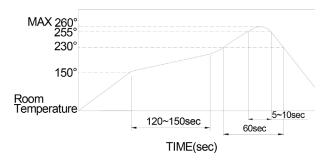
The condition mentioned above is the temperature on the Cu foil of the P.C.B surface. There are cases where board's
