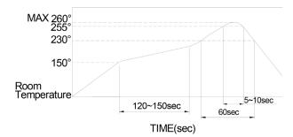
The condition mentioned above is the temperature on the Cu foil of the PCB surface.
