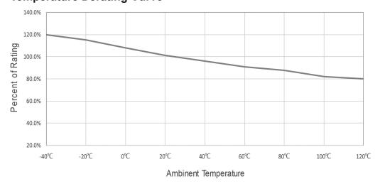
Calculation for ideal fuse selection =  $\frac{Operating Current(A)}{Rating \times 0.75}$
