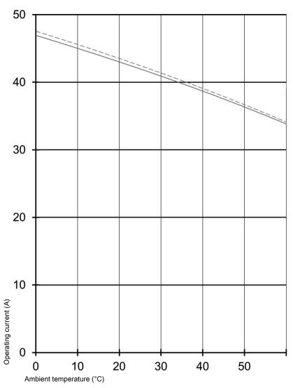
\_ \_ 4 mm² (female side) and 10 mm² (male side) \_\_\_ AWG 12 (female side) and 10 mm² (male side)
