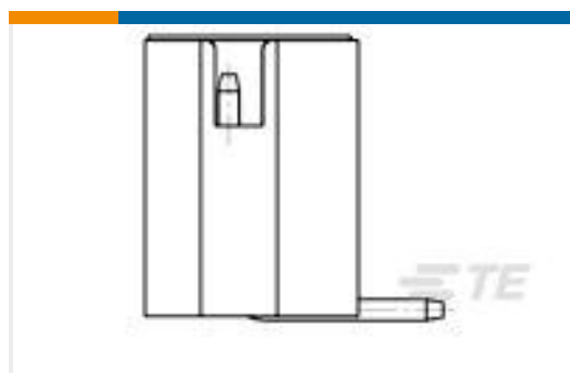
TE Part #1775470-8 HPI CONN., 2.0MM, V/T, SMT, 8P, 80U"
