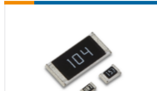
TE Part #4-2176343-8 CRGCQ 1206 82K 1%
