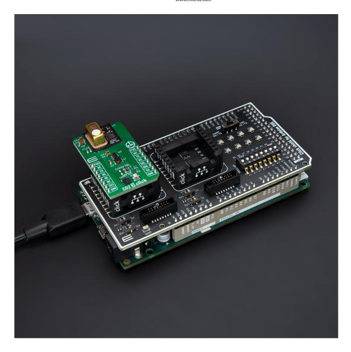
When the USB is connected to the Arduino DUE board, the PWR diode will glow Green, and at this setup, the Arduino DUE baseboard itself will be supplied, and it will provide power to the Click Shield, including all mikroBUS $^{\text{TM}}$  sockets.
