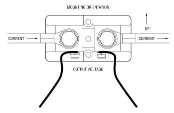
**Operating Current Derating:** For continuous operation, it is recommended that shunts are not operated at more than two thirds (2/3) the rated current under normal conditions per IEEE standards for DC instrument shunts. At ambient temperatures above 40 °C, the current must be further derated to prevent damage.
