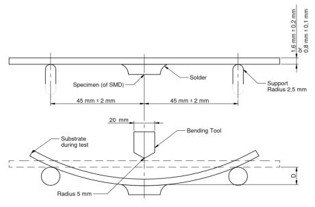
This substrate bending test is for all size of WCAP-CSST.
