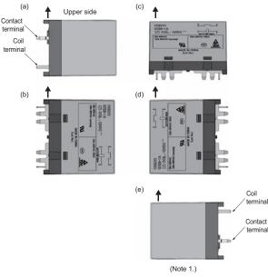
Note 1. The operating voltage differs from the applied coil voltage for contact terminals mounted in the downward direction (e). Please refer to ●Coil on page 2 and ●Coil Voltage Reduction (Holding Voltage) during and after Relay Operation.
