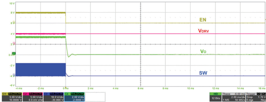
Fig. 25 - Shutdown with EN, 25 A load
