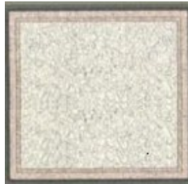
Figure 6 - Micro photography of a 100pF Capacitor
