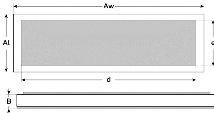
Figure 3 - Package outline 4.7nF Capacitor
