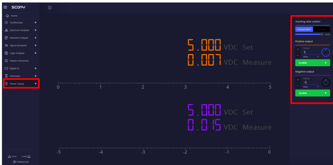
Figure 21. Setting the Supply Voltages in Scopy for the Capacitive Load Stability Demo
