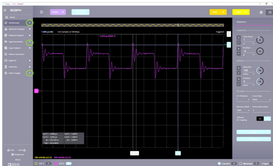
Figure 25. Expected Channel 2 Output Waveform – J2 Jumper Installed
