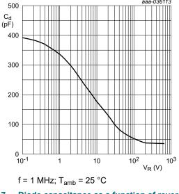
Fig. 7. Diode capacitance as a function of reverse
