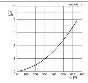
Fig. 8. Capacitance stored energy as a function of reverse voltage; typical values
