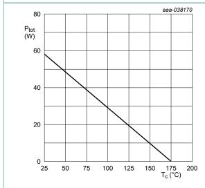
Fig. 2. Power dissipation; maximum values
