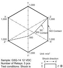
applied in  $\pm X$ ,  $\pm Y$ , and  $\pm Z$ Z' 🚫 directions three times each with and without energizing the Relays to check the number of malfunctions.
