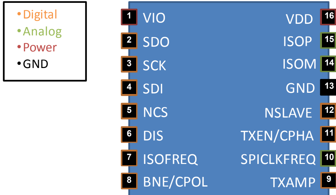
Figure 2. Pin connection diagram (top view)
