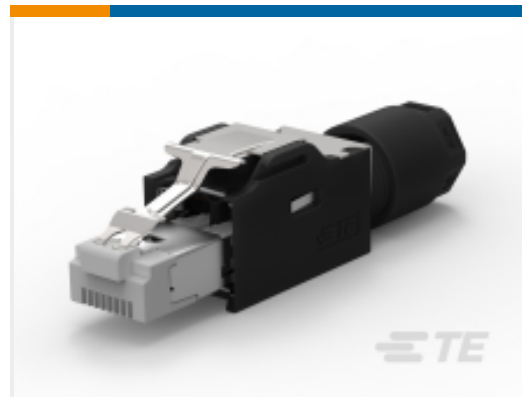
TE Part # 2120892-1 RJ45 CONNECTOR CAT6A, IP20 PLUG
