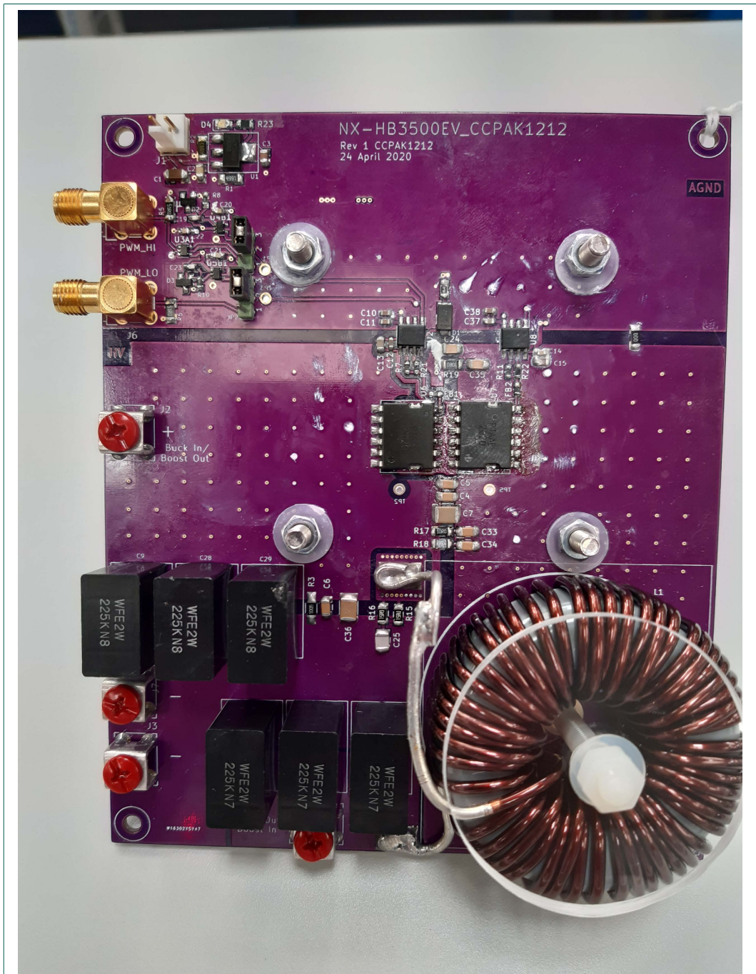
Fig. 3. NX-HB-GAN039-BSCUL bottom-side cooled half-bridge evaluation board
