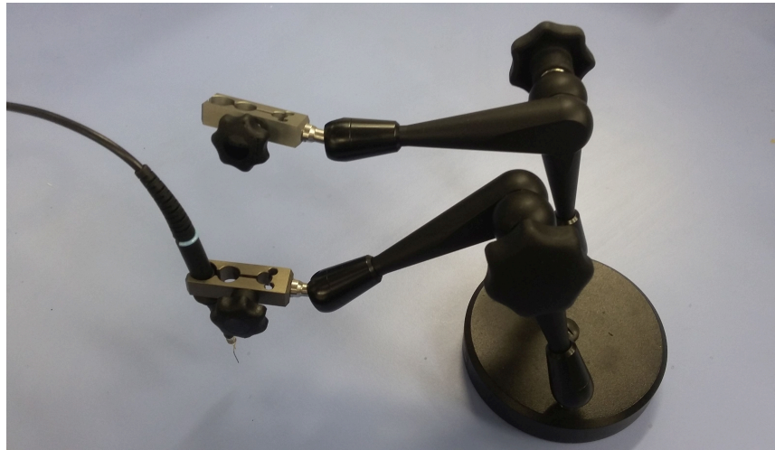
Fig. 2. Example of a probe positioner
