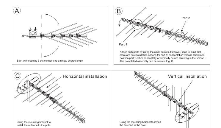
Using the mounting bracket to install the antenna to the pole.
