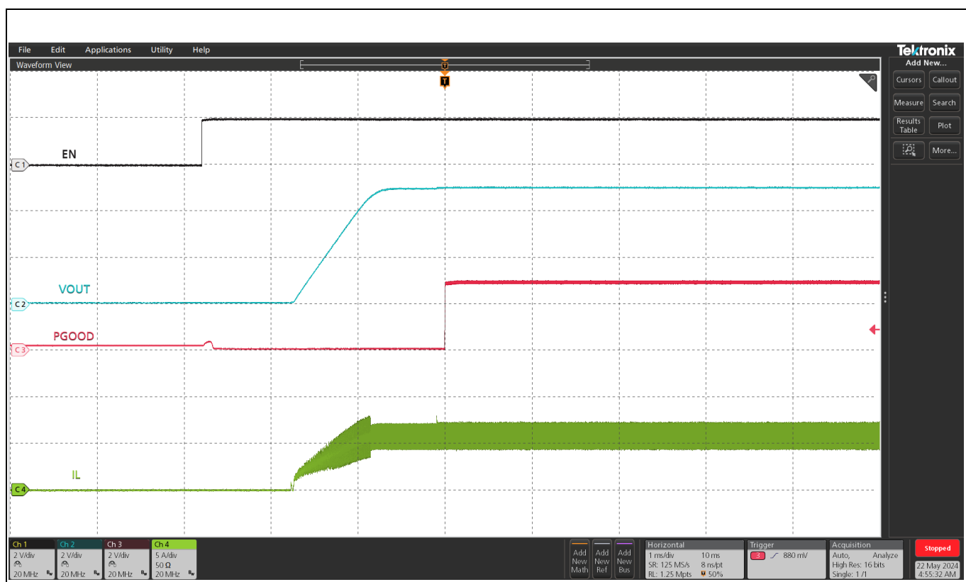
Figure 9 Start up at 6A Load, (Ch1: Enable, Ch2: Vout, Ch3:PGood ,Ch4: Inductor Current)
