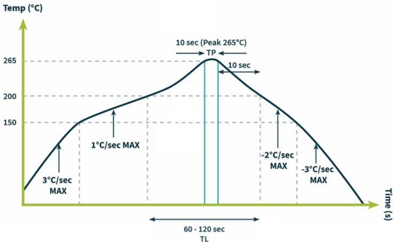
\*Temperatures listed within a tolerance of +/- 10° C
