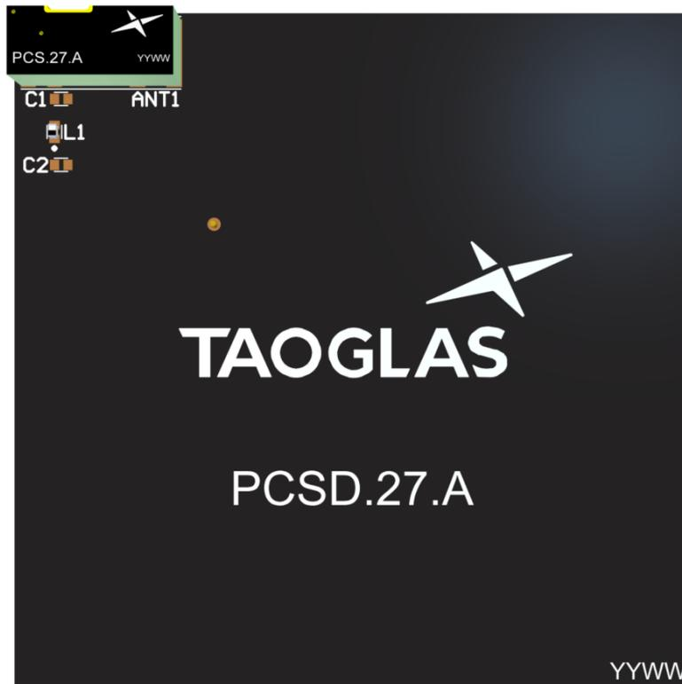
Above is a 3D model of the PCS.27.A on a PCB.
