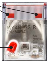
Relay with AC Coil (LED: Red)
