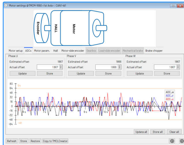
Figure 8: Configuring the Motor Current ADCs
