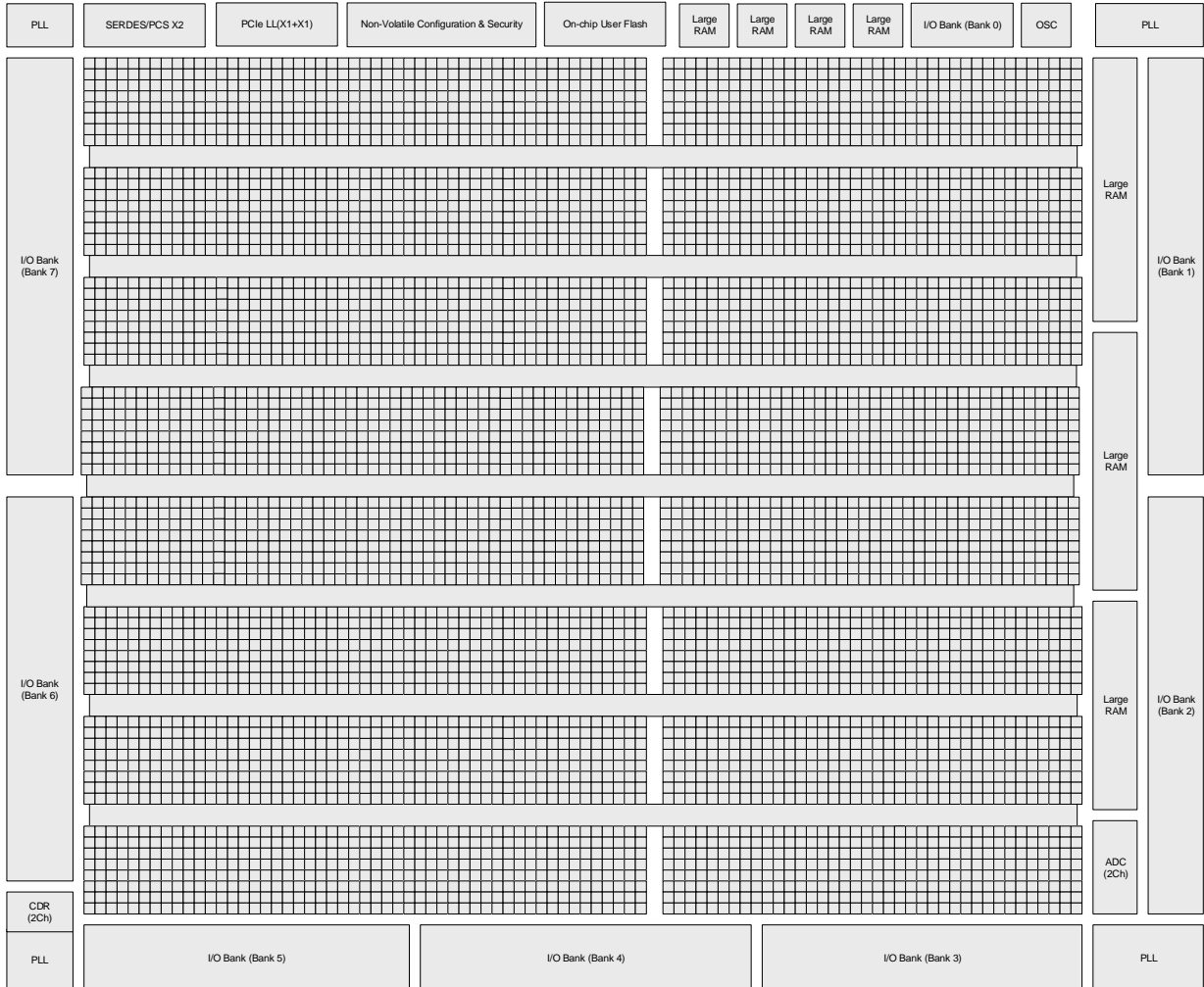
Figure 2.2. Simplified Block Diagram, MachXO5-NX-55T Device (Top Level)
