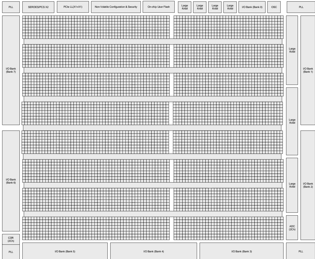
Figure 2.3. Simplified Block Diagram, MachXO5-NX-100T Device (Top Level)
