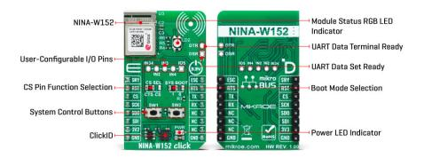
Security is a key feature of the NINA-W152. It supports secure boot, ensuring the module only operates with authentic u-blox software. Additionally, it provides robust end-to-end security on the wireless link, utilizing the latest 802.11i standards (WPA2/WPA3) and enterprise security protocols, making it ideal for secure IoT applications in telematics, industrial automation, connected buildings, wireless sensors, point-of-sale systems, and medical devices.
