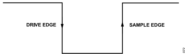
Figure 72. SPI Mode 3, SCLK Edges
