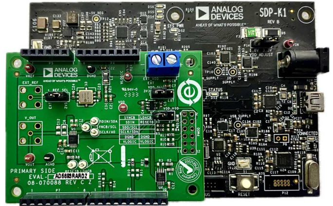
Figure 1. Evaluation Board Connected to the SDP-K1 Controller Board (EVAL-AD5683RARDZ or EVAL-AD5693RARDZ Version)
