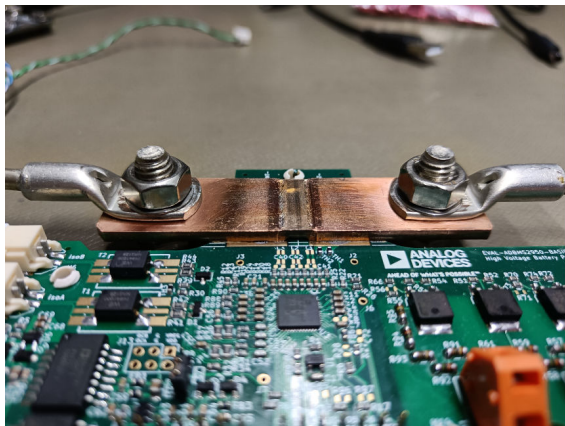
Figure 17. Attaching Cable Lugs to Shunt Resistor, Part 2
