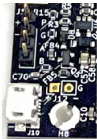
Figure 21. Connectors Options on EVAL-ADBMS2950B Evaluation Board
