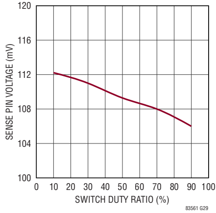
SENSE Current Limit vs Duty Ratio
