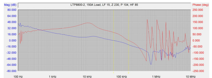
Figure 3. Measured Bode Plot of the LTP8800-2
