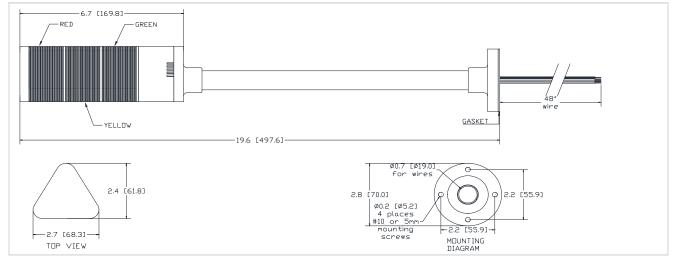
LED OPERATION: | CONNECT STACK COLOR WIRE TO POWER AND BROWN WIRE TO POWER.
