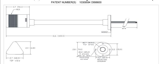
LED OPERATION: CONNECT STACK COLOR WIRE TO POWER AND BROWN WIRE TO POWER.
