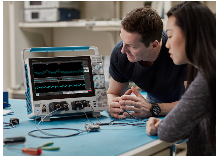
Voltage measurements on a switch-mode power supply showing the ripple voltage on one of the power rails.
