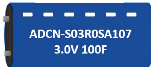
Example of the Markings of a 100F 3.0V capacitor
