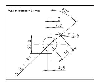
Optional, the sensor can be mounted with a standard Delphi-clip.
