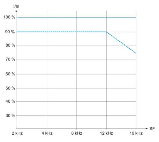
40 °C (104 °F) - Mounting type A and B 50 °C (122 °F) - Mounting type A and B In : Nominal Drive Current
