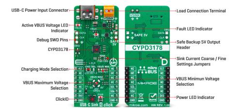
The CYPD3178 on the USB-C Sink 4 Click supports multiple charging protocols. When connected to a non-PD charger, it can negotiate with any legacy charging protocol supported by the sink device. The CHG SEL jumper allows users to configure the supported protocols. The jumper is set to the LGC position by default, enabling support for all legacy charging protocols. However, by switching the jumper to the BC1.2 position, the device limits its operation to the BC1.2 charging protocol only.
