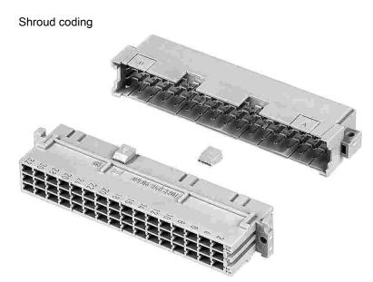
Insert the code key into one of the key ways of the female connector as shown in the drawing. Break out the corresponding area of the male shroud. Connectors coded this way can only be applied in a minimum rack spacing of 20.32 mm.
