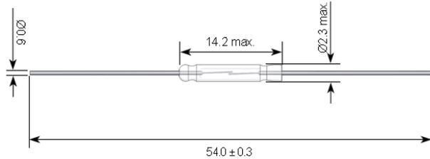
tolerances according to DIN ISO 2768 m
