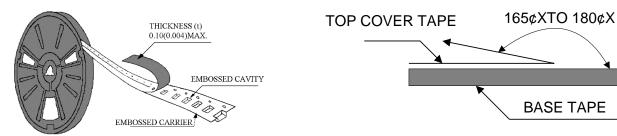
The force for peeling of cover tape is 10 grams in the arrow direction.
