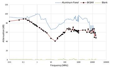
Test performed with a two-coat thickness.
