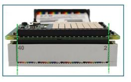
1.Insert 40pin black male connector into 40pin female connector at the back of Pi 400. If black male connector can't be inserted into Pi 400, the orientation of the black male connector is wrong, please reverse the cable and re-insert.
