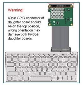
3.Please double check the orientation of daughter board and position of pin#1,2 & 40 base on the below chart before power on Pi400.
