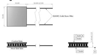
Ceramic Material: Al<sup>2</sup>O<sup>3</sup> / Solder Construction: 232°C, SbSn
