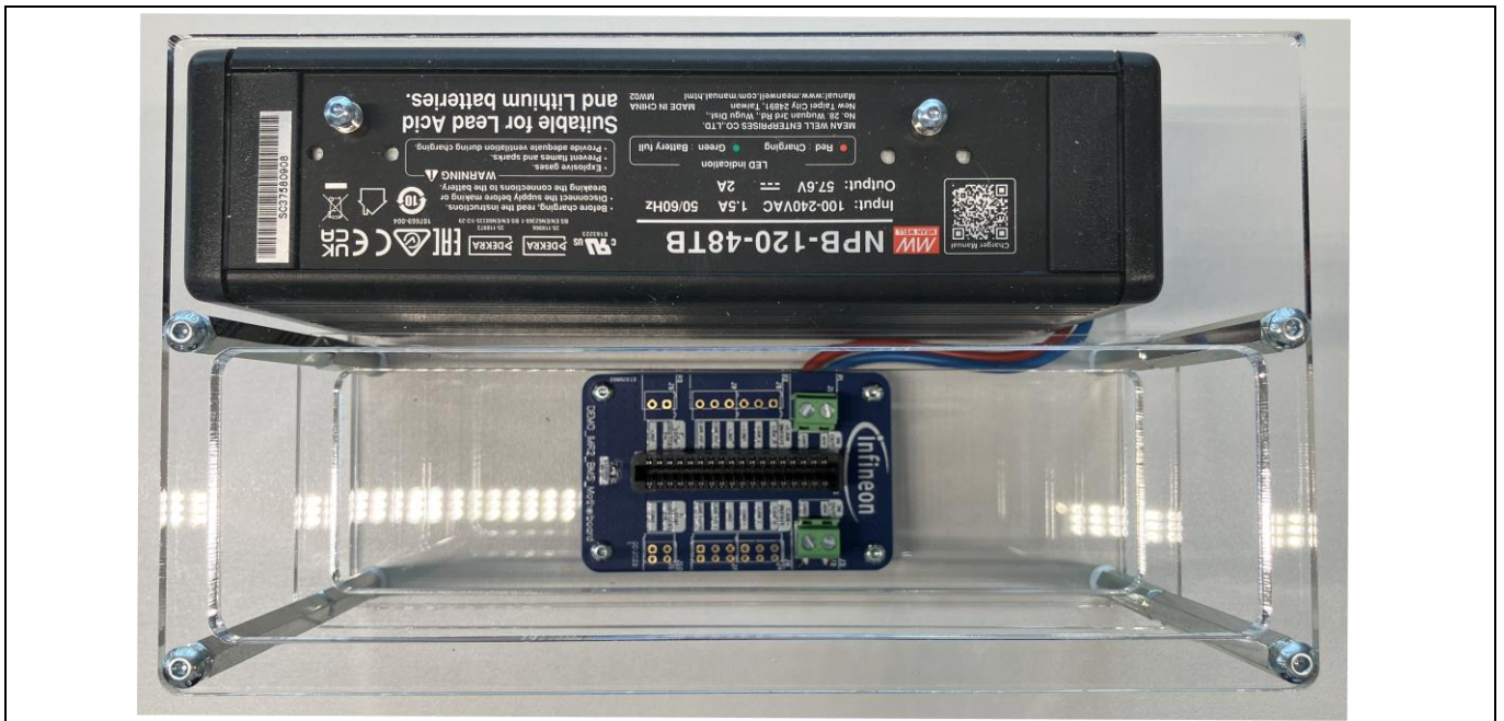
Figure 22 Recharging onboard batteries in the external charging unit (charging)
