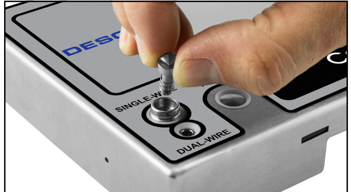
Figure 6. Inserting the plunger and spring assembly into the single-wire jack
