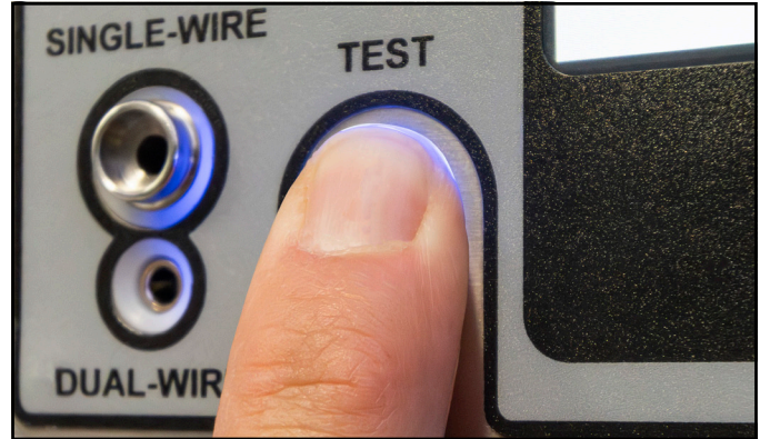
Figure 25. Bridging the test switch's contacts
